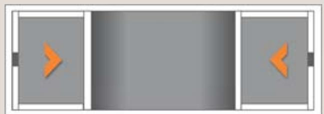
TD10 Three-panel sliding door with two (side) active panels
